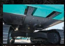
Upper Under Covers Thick covers with increased durability compared to SK500HDLC-8. \$1520
